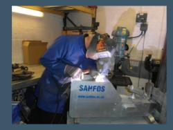
Chris Harris, who is an expert boiler maker by trade, is carrying out stainless steel welding repairs to a CPR that was damaged whilst being recovered in rough weather.
